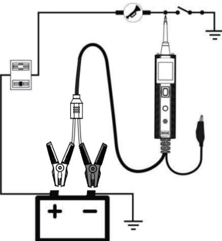
► With this function, if you are contacting a protected circuit, a vehicle's fuse can be blown or tripped if you apply ground to it.
