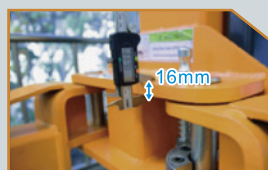
16mm thickened steel plate
