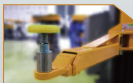
Standard with three-stage screw pads and height extension sleeve
