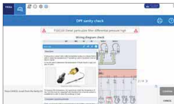
Other diagnostic procedures to support troubleshooting, such as wiring diagrams, technical sheets or additional useful information.
