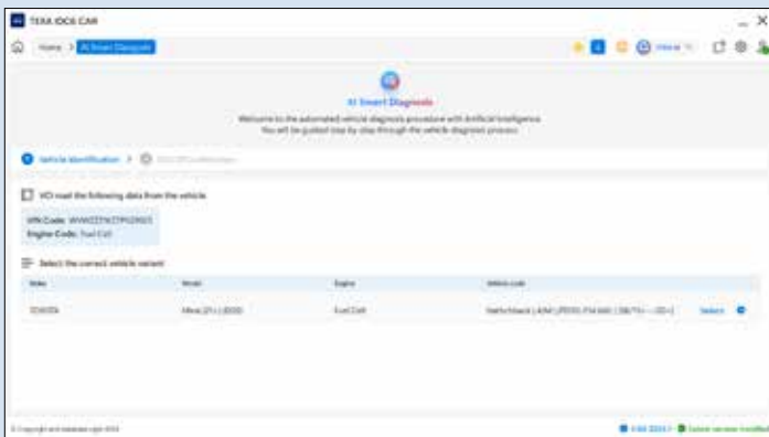
Possible request to specify more precisely the type of vehicle, displayed only if the automatic identification is not sufficient to identify the vehicle univocally.
