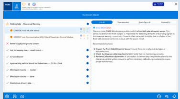
In the left part of the screen all the control units scanned in the vehicle are displayed, whereas in the right part there is the information on the selected control unit. The information is organised in tabs.
