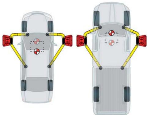
It combines the advantages of an asymmetric and a symmetric lift and improves the ergonomics when placing the arms to lift the car
