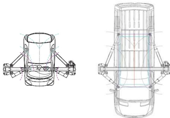
Thanks to the Versymmetric® Technology vehicles with short (i.e. Smart) as well as long wheel base (i.e. mid size vans) can be lifted comfortably
