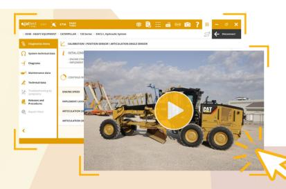
Motor graders are machines used in land levelling tasks, hence the need for all the elements used to carry out these levelling tasks to be well calibrated and adjusted. Wear or replacement of the articulation and steering position sensors requires their calibration to obtain a correct detection of the machine positions, thus achieving greater performance and working precision.
