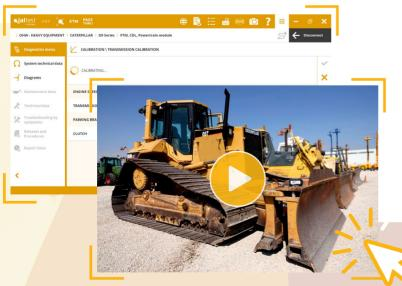
This type of machines use the powertrain as steering and displacement system. Wear or replacement of the powertrain components requires its calibration to obtain a greater precision during forward and displacement, thus achieving greater comfort and performance at any speed, as well as a linear displacement without deviation of the machine.
