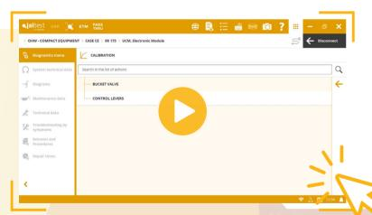
This machine has two Joysticks with electronic control to manage the hydraulic system and the propulsion system. Wear or replacement of these components requires their calibration to obtain a smooth operation at the exact moment, thus achieving greater comfort and performance at any speed.
